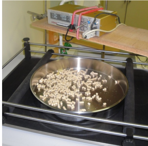
Figure 2.16. Mechanical shaker and Grimm 1.109 spectrometer (Grimm Aerosol Technik GmbH & Co. KG, Airing, Germany), without the weatherproof housing, used for the shake test. From each diet, 100 g was shaken for 20 min.
