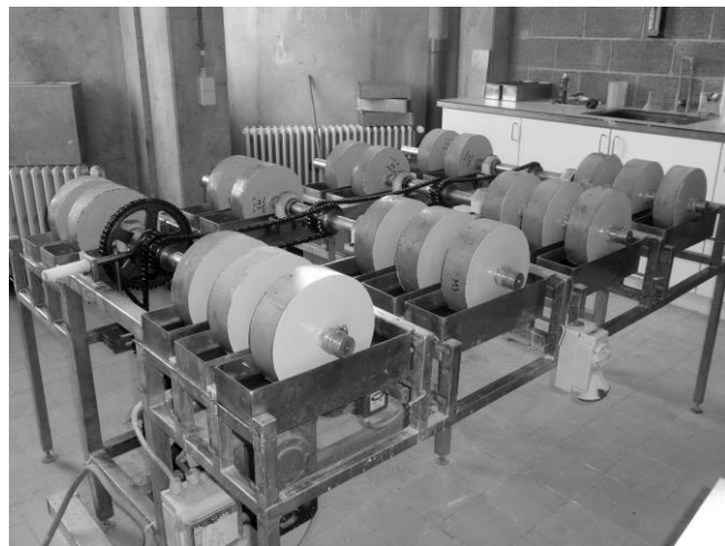
Figure 3.6: The test set-up for cyclic immersion and drying test.
