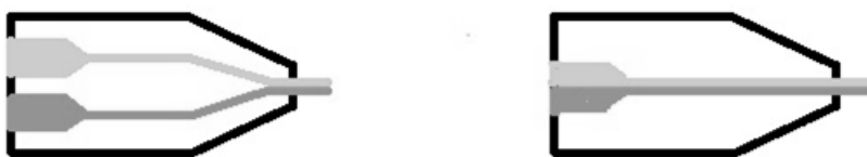
Figure 2. Schematic representation of a multimanifold die (left) and a single-manifold die (right).
