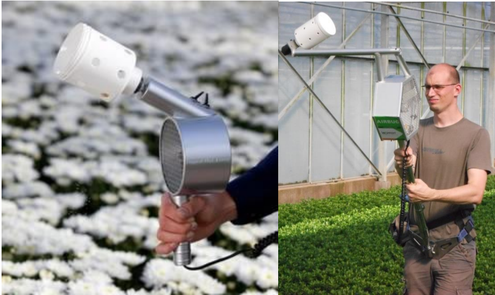
Figure 1.12: Mini-airbug and Aerobug marketed by Koppert B.V. to distribute predatory mites in the crop (left: Koppert, 2015; right: Photo author)
