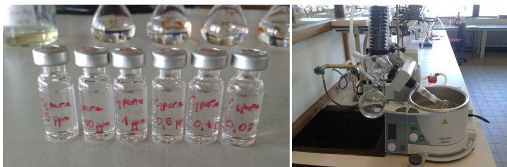
Fig. IV.2: a) Standard solutions of cypermethrin to perform the calibration and quantification line. b) Setup of evaporation to concentrate the extract.
