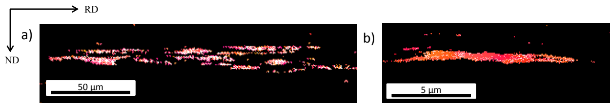
Figure 4-26: Deformed cube grains after 90% deformation (a) RT, (b) cryogenic. LAGB are depicted in white.
