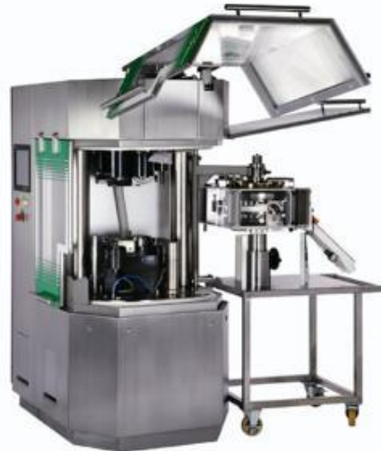
Figure 2.1: The Modul TM P, with the ECM removed from the machine. (Courtesy of GEA, Courtoy TM )
