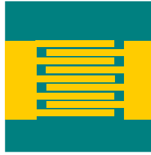
Figure 2.21: A sketch of the structure of a MSM, yellow indicates metallisation, blue the semiconductor substrate (InGaAs in our case).
