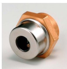
Figure 2.20: The external view of a G4176-03 MSM photodiode, which was used during this work. Copyright Hamamatsu Photonics.
