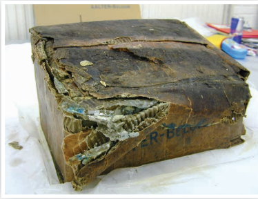
Fig. 43 Joseph Beuys: Butter and beeswax, basic material 4/b , degradation of cardboard due to fat impregnation.
