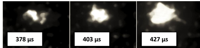
Figure 7.8: Succeeding time-resolved images of the initial stage of combustion. Indicating cool- and hot flame ignition. t = 378\mu\text{s} (cold flame ID), t = 403\mu\text{s} , t = 427\mu\text{s} (hot flame ID) = t_{ign}
