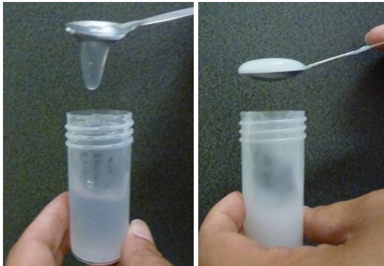
Figure 3-5: Translucent long texture of waxy maize starch paste (5:100, no xanthan) heated to 85°C (L) and short opaque paste (R) heated to 70°C (5:100, no xanthan)
