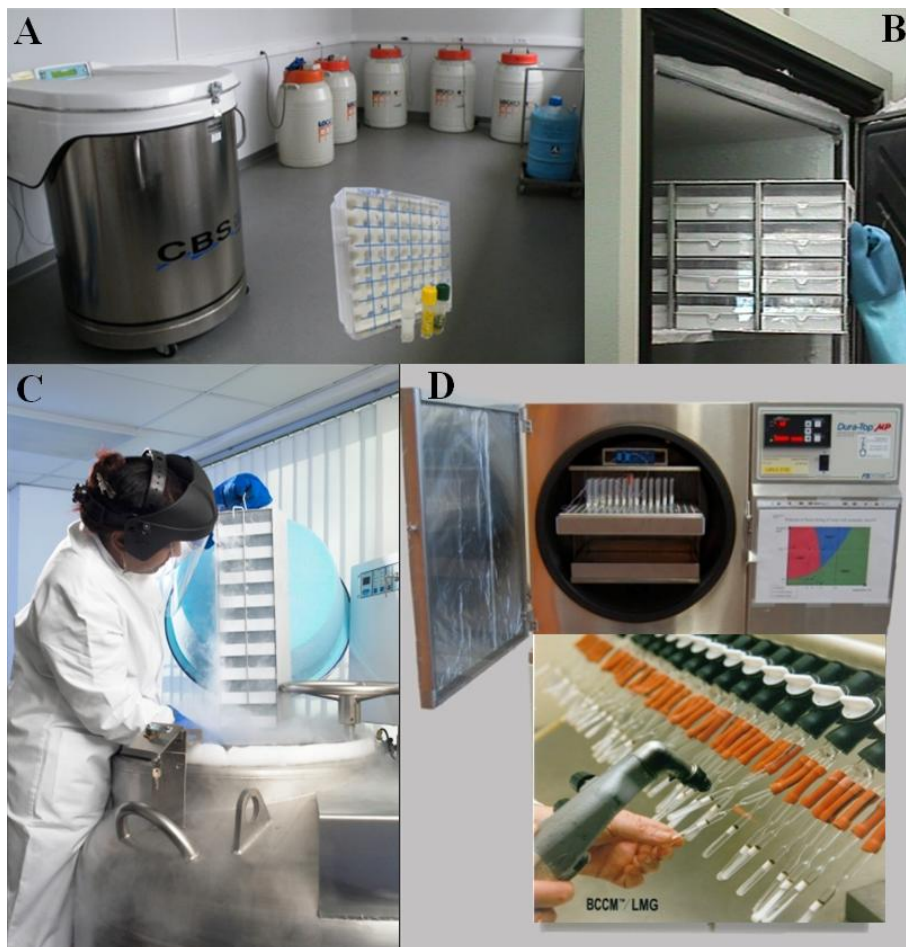
Figure A-4: Liquid nitrogen containers, cryotubes, and racks for cryopreservation at temperatures below -135^{\circ}\text{C} (A, C). Cryopreservation at -80^{\circ}\text{C} in electrical freezers (B). Lyophilization equipment and freeze-dried ampoules (D). Pictures obtained via the BCCM LMG Bacteria Collection.
