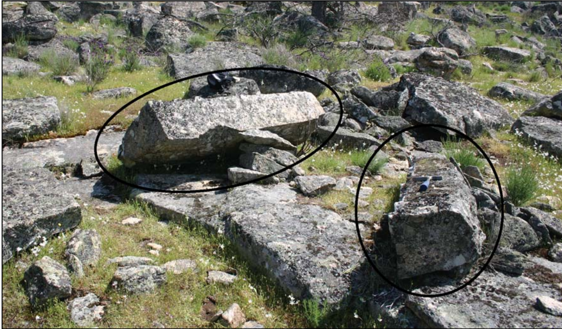
Figure 8.19 Two blocks from the same 'core' block separated using wedges. Traces of used wedge sockets can still be seen on the right block (length hammer: 30 cm) (location: 39.370881° N, 7.313383° W (WGS84)).
