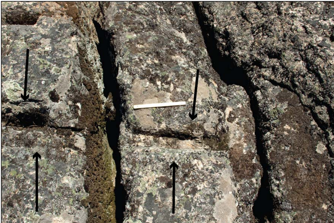
Figure 8.17 Shallow channel for placing wedges and guiding the splitting (scale: 20 cm) (location: 39.369034° N, 7.313209° W (WGS84)).
