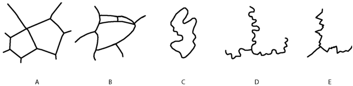
Figure 9.3 Grain boundary shapes according to Collerson (1974): (A) straight, (B) curved, (C) embayed, (D) sutured, and (E) serrated.
