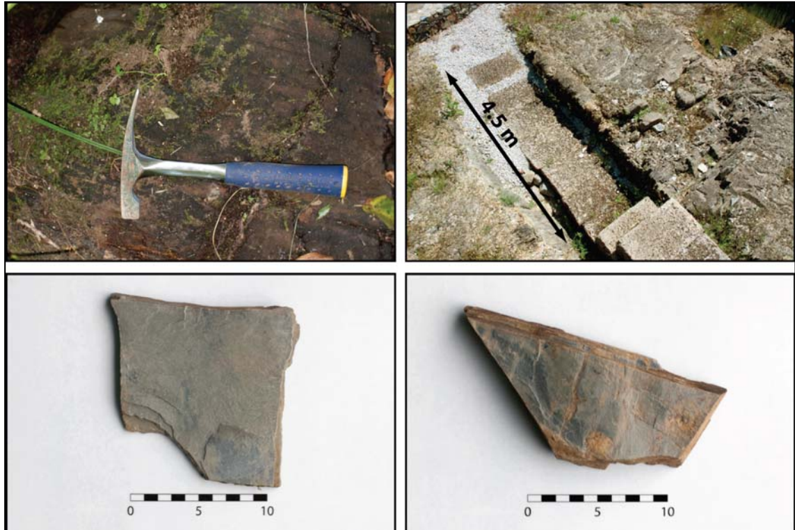
Figure 7.10 Shale outcrops near Ammaia : (A) Shale bedrock in the Sever riverbed (length hammer: 30 cm); (B) Hand specimen of the dark grey shale from the Sever riverbed; (C) Foundations of mausoleum in the suburban area between the town and the Sever River dug into the shale bedrock; (D) Hand specimen of the dark grey shale from the suburban area.
