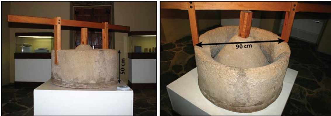
Figure 5.6 Ring- catillus mill from Ammaia .
