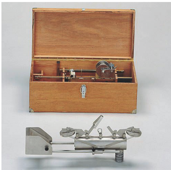
Figure 2.10: Watertrap sampler (Eijkelkamp, 2012)
