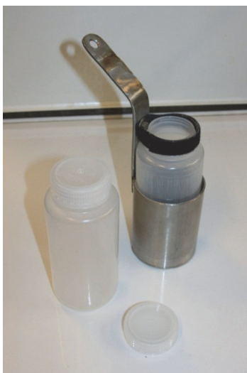
Figure 2.2: Weighted-bottle sampler as constructed by FHR
