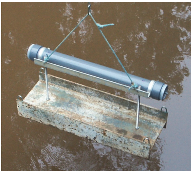
Figure 2.15: Time-integrated sampler (TIS) as constructed and deployed by FHR
