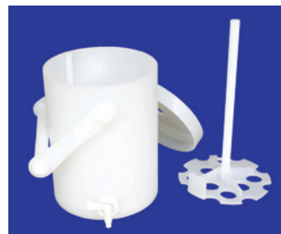
Figure 2.8: Churn sample splitter (FISP, 2011)
