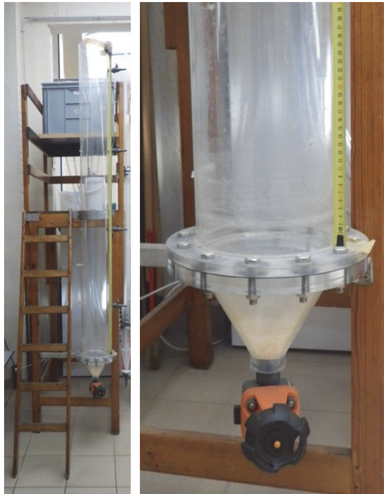
Figure 3.5: Settling tube constructed in FHR's sedimentological laboratory
