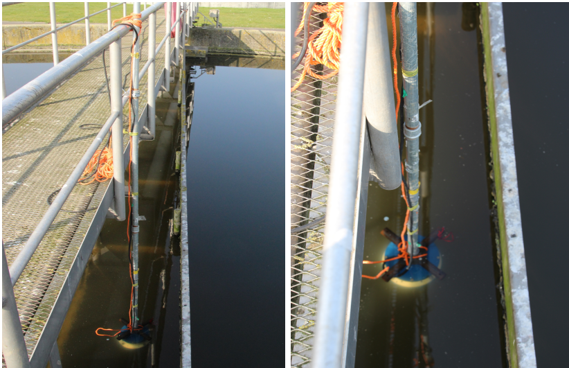
Figure 8.13: The experimental set-up of the ADCP
