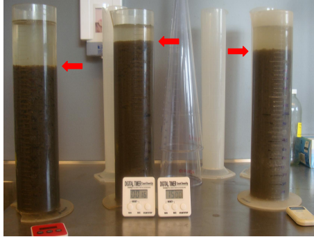
Figure 5.1: Photograph of a batch settling tests indicating the suspension/liquid interface
