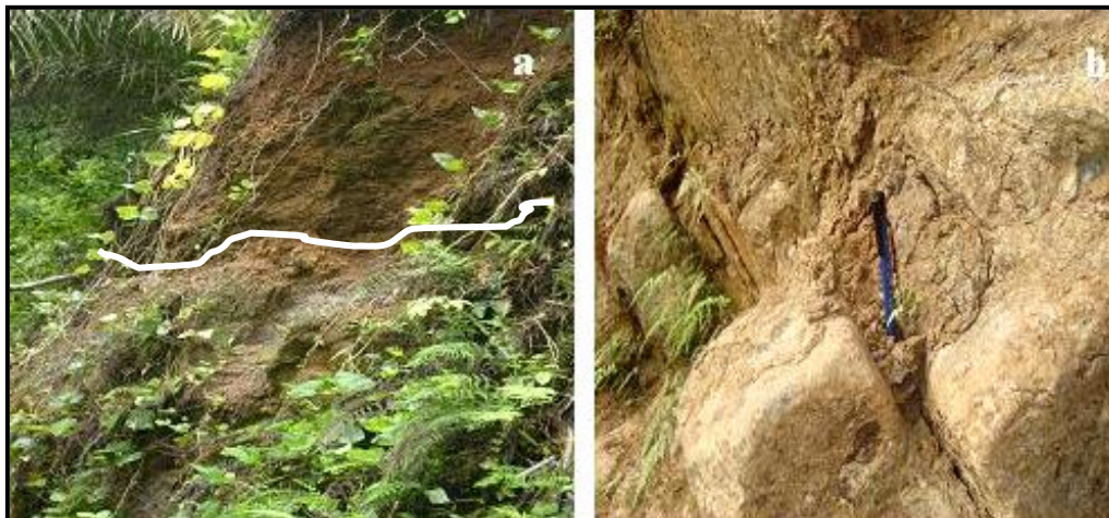
Fig. 2. 8. Contact between soils and saprolite and the characteristics observed at the head scarp: a) reddish brown soils and underlying gray saprolites at slide 8 Makuka; b) jointed basaltic blocks at head scarp of a rotational slide at Bonjo sandwiched by pale yellow clayey soils.
