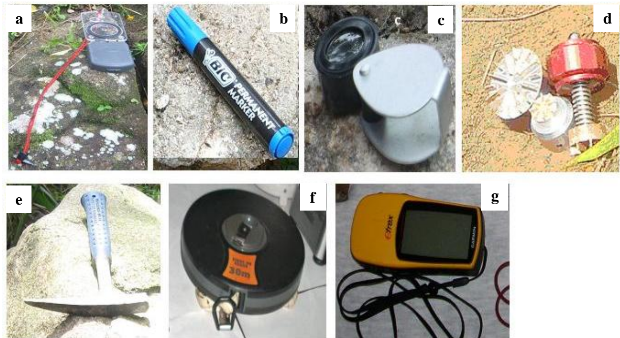
Fig. 2. 3. Catalogue of equipment used in the field; a) Silva compass clinometer for orientation and inclination measurements; b) Permanent bold marker used in the labelling of samples; c) Hand lens; d) Torvanometer used to measure in situ relative shear strength of the soils; e) geologic hammer; f) Measuring tape; g) Etrex Garmin GPS receiver.
