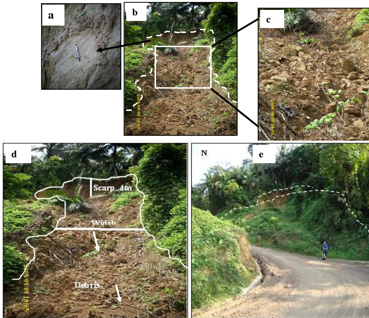
Fig. 2. 17. Field view of 2008 reactivation of the Bonjo slide; a) slicken slide at the head wall; c) detailed view slide debris; d) view of the 2008 reactivation of the 2005 Bonjo slide a week after slide reactivation. e) View of the July–August 2008 slide (photograph taken in November 2008). Note the backward migration of the head scarp and the degree of re-vegetation of slide debris three months after reactivation.
