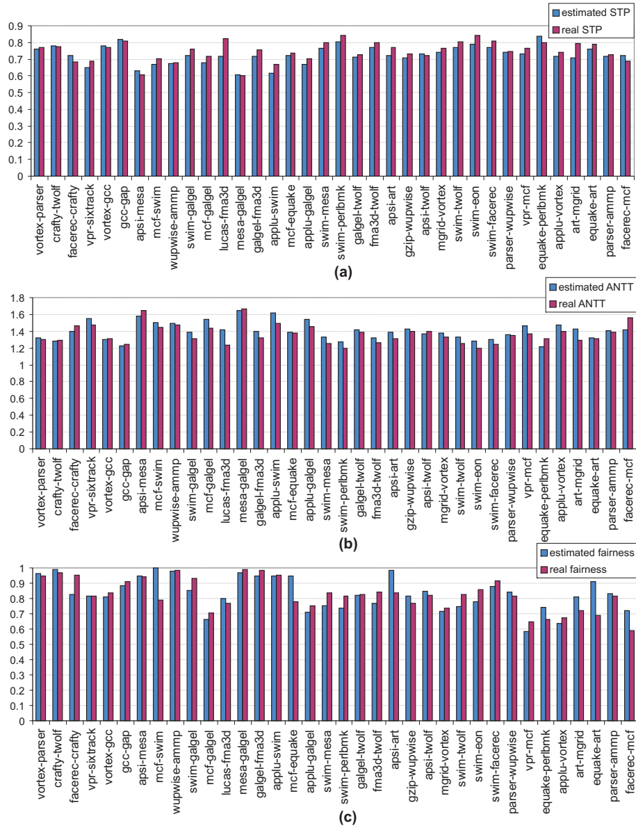
Figure 6.13: STP (a), ANTT (b) and fairness (c) values, predicted by the cycle accounting architecture, compared to the real values (calculated using post-execution single-threaded simulations), assuming dynamic resource partitioning and the ICOUNT fetch policy.
