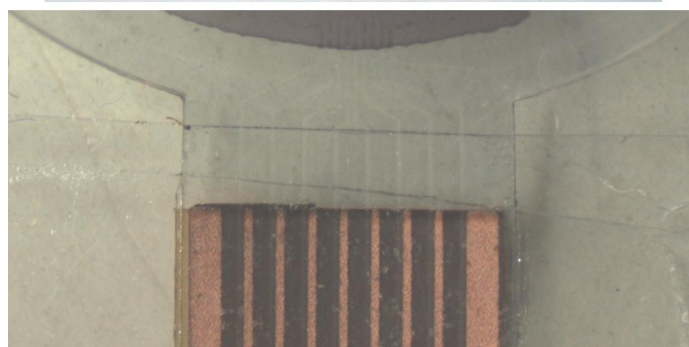
Figure 6.5: New flexible connector. Top: Copper clad laminate patterned on both sides. Yellow areas is polyimide, orange areas is copper at the top surface, dark areas is visible copper at the backside. A multitude of connectors was designed and usually comprised a long narrow rectangular part and a fan-out. Bottom: Close-up of a connector that was inserted and carefully aligned with the PEDOT:PSS tracks at the rectangular contact areas of the LC cell.
