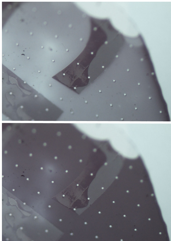
Figure 4.16: Patterned LC cell using the scanning technique. Top: The voltage off state reveals the LC molecules did not align properly in the ablated areas and sometimes the square mark of a single pulse could even be discriminated. Bottom: When applying a voltage and thereby switching the cell it was confirmed that the PEDOT:PSS was sufficiently removed.
