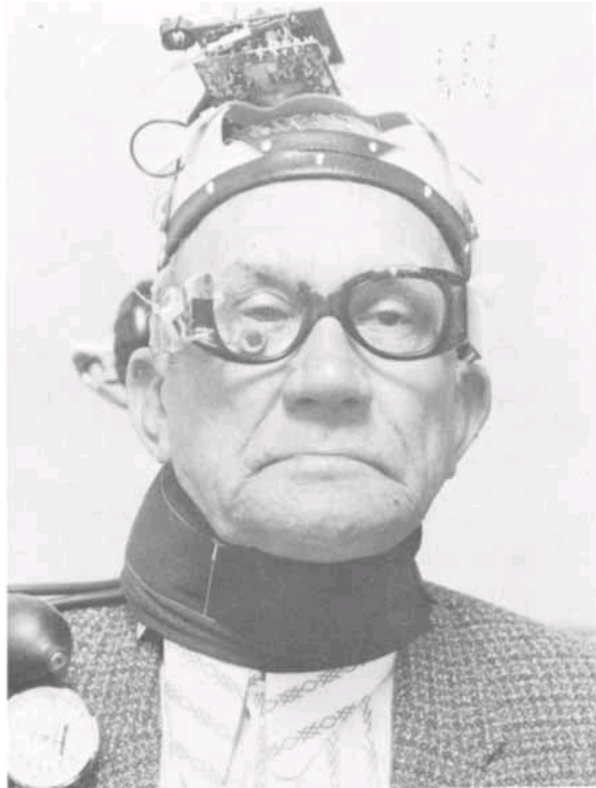
Figure 2.3: Complete set-up as used by Cooper et al. [7] in 1983 to detect IOP.
