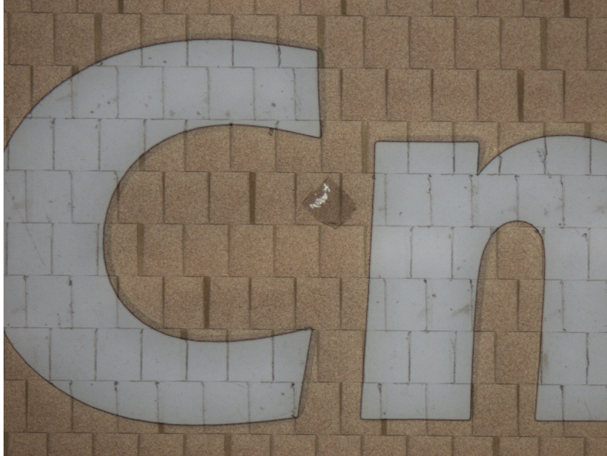
Figure 4.13: After developing a patterned photoresist on top of the PEDOT:PSS, a laser with a 200 by 200 \mu\text{m} square beam shape is scanned across the surface, thereby ablating both the top layer of the photoresist as the PEDOT:PSS layer. In the middle of the picture a ablated PEDOT:PSS flake can be seen, which is washed away in a subsequent step.
