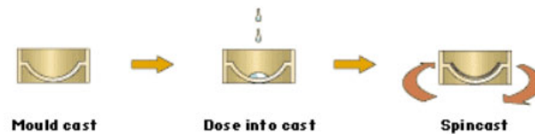
Figure 1.10: By casting some unpolymerized material in an open, spinning mold, a contact lens with a spherical back surface can be created. Image from [23].
