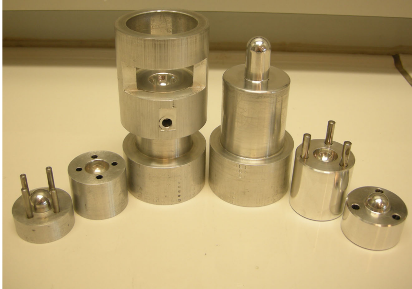
Figure 4.7: Three generations of molds. On the left the first mold used for our first prototype, in the middle a CNC fabricated mold which was deemed unpractical due to its size and on the right the third generation mold with carefully tuned dimensions.
