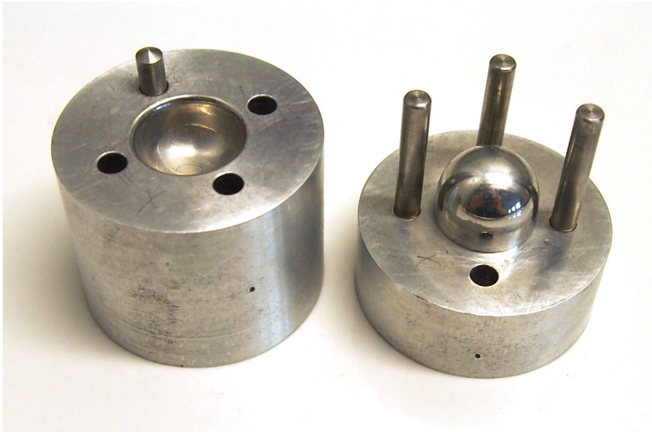
Figure 3.7: Mold comprising 2 parts: a male, convex side and a female, concave side. Both are made of aluminium and have a radius of 7.8 mm. 4 guiding pins are foreseen to ensure a correct placement of the two parts and prevent rotation vis-a-vis each other while the cells are being molded.
