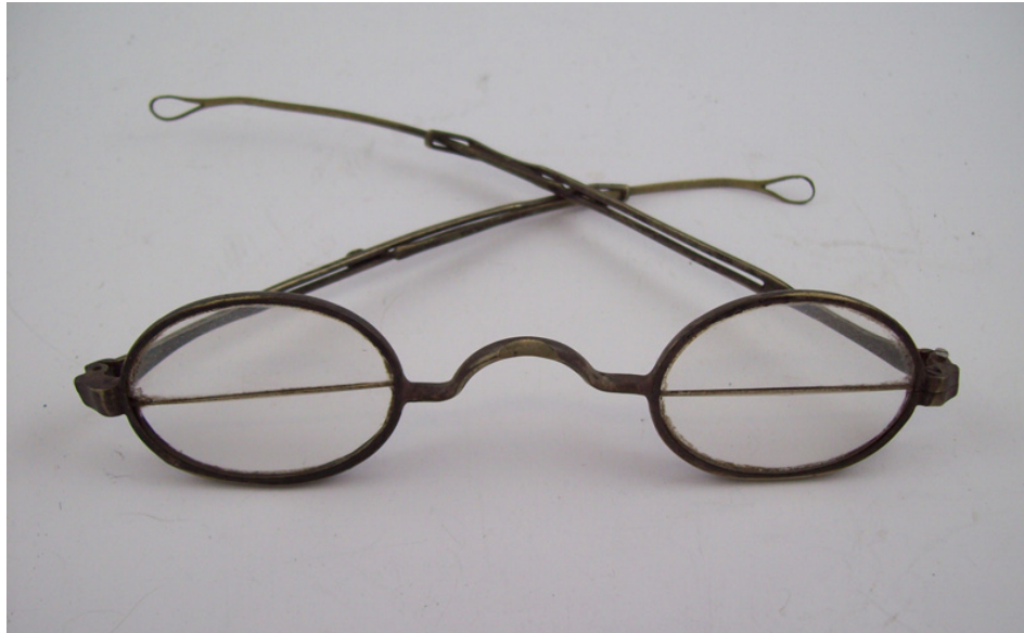
Figure 1.8: A typical example of early bifocal glasses. Depending on the viewing angle, the wearer can select a lens to either read at close point or to look at objects at a distance.
