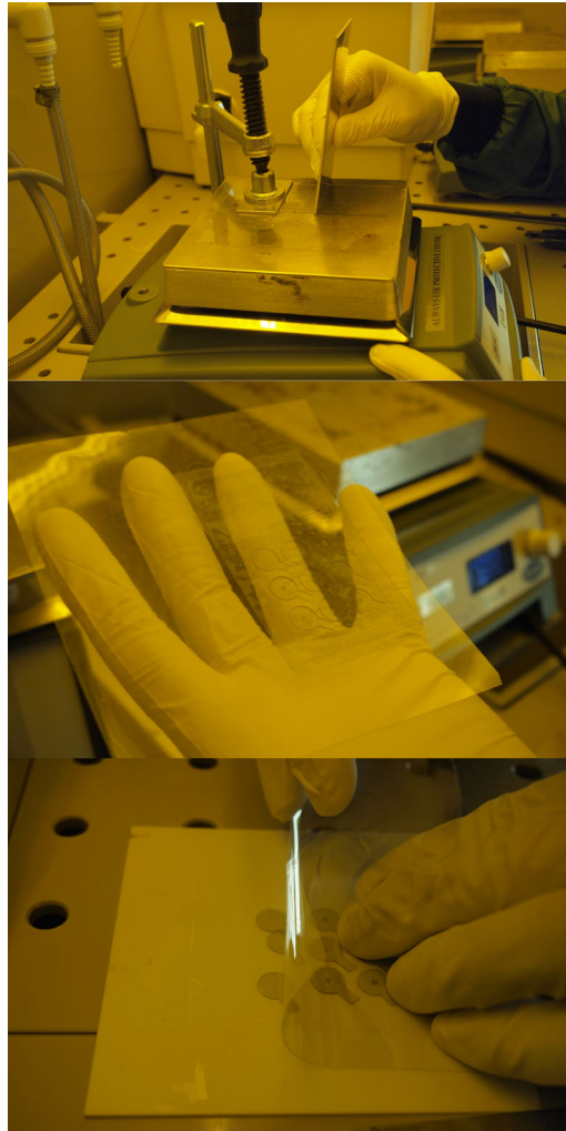
Figure 3.15: Transfer-to-Foil Method. Top: the bottom carrier glass is removed using the conventional method after clamping the stack on top of a carrier foil. Middle: after delamination the carrier foil containing the redundant part of the glued PET-films and the laser cut LC cells can be peeled off from the hot plate. Bottom: the LC cells can be manually picked from the carrier foil or can be transferred en masse to a new rigid carrier.
