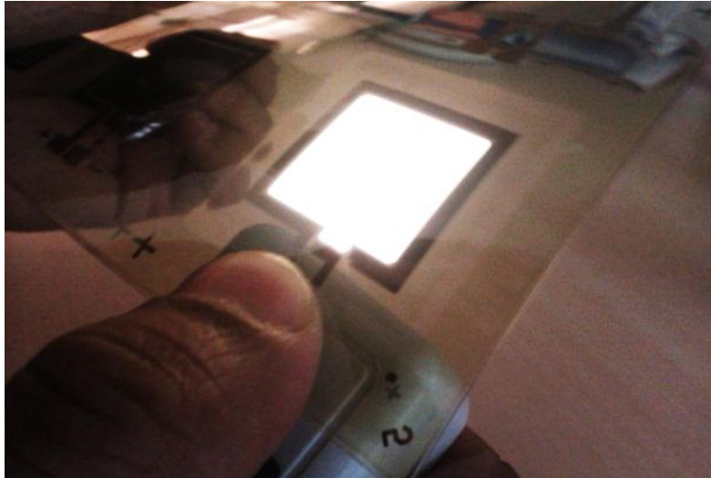
Figure 4.12: A functional flexible OLED device incorporating PEDOT:PSS and LEP selective ablation using excimer laser, demonstration under environmental conditions.
