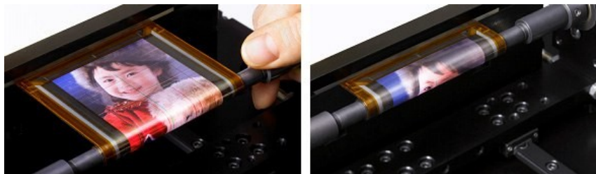
Figure 1.2: Demonstration of a 4.1" prototype flexible display from Sony: Ultra-thin OLED screen could continue to play video while being rolled around a pen [25].
