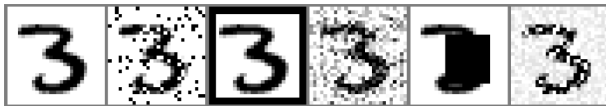
Figure 8.2: From left, a clean MNIST sample and its corresponding noisy versions which are salt & pepper, border, Gaussian, block, and speckle, respectively.
