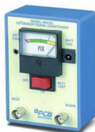
Figure 3-17: Photograph of the signal conditioner of type 480C02 from PCB Piezotronics [22]
