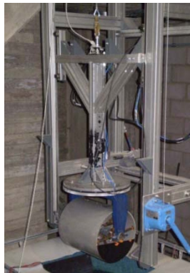
Figure 3-21: The complete impactor including the stiffened cylindrical test object
