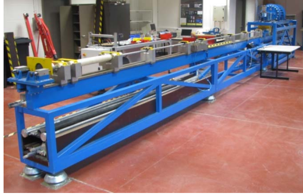
Figure 4-24: Photograph of the used split Hopkinson pressure bar test setup
