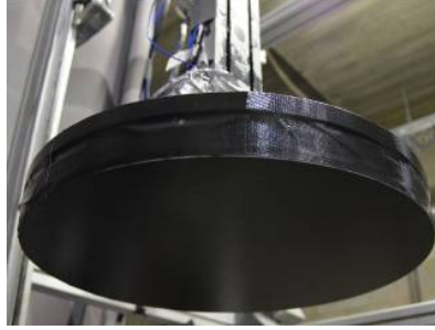
Figure 3-26: Photograph of the impactor plate combined with a PVC plate as being a rigid flat plate test object
