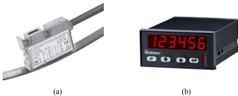
Figure 3-12: Photograph of the position encoder (a) and its corresponding counter device (b) [14]
