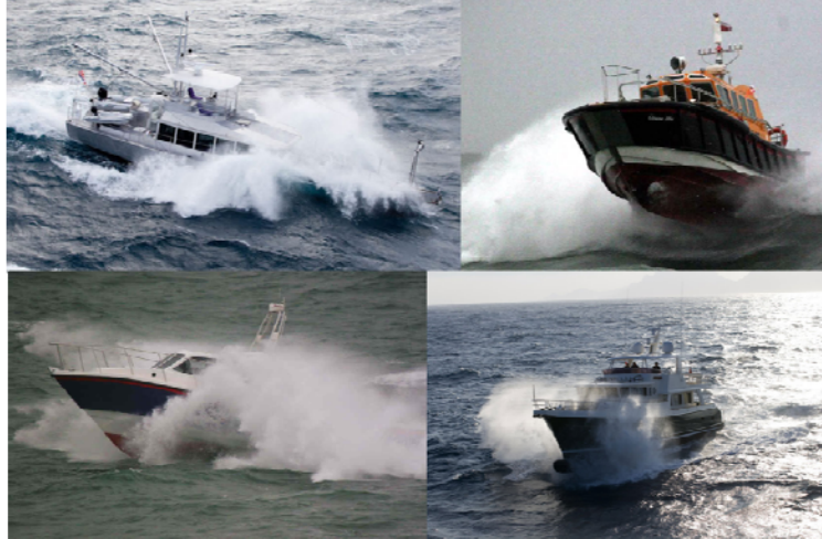
Figure 2-1: Pure bottom slamming of small vessels
