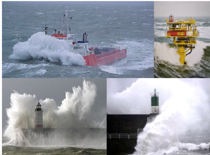
Figure 2-4: Examples of pure breaking wave slamming
