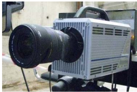
Figure 3-14: Photograph of the Photron APX-RS high speed camera
