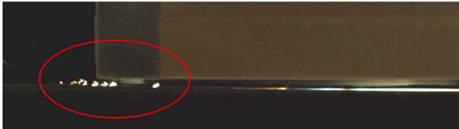
Figure 6-6: The presence of initial surface waves before the water impact of a flat plate [2]
