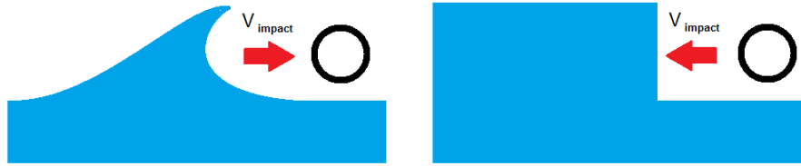
Figure 1-7: The real slamming situation compared to the experimental approach for breaking wave slamming
