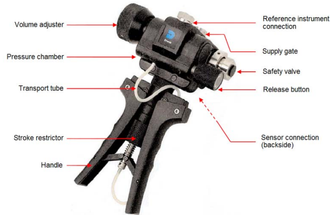
Figure 4-17: The pressure hand pump for static calibration of pressure sensors
