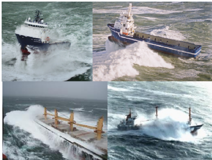
Figure 2-2: Pure bottom slamming of large vessels
