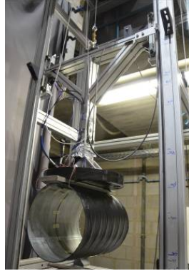
Figure 3-25: The impactor containing the GFRP cylinder with D = 32.17 cm and d = 3.325 mm
