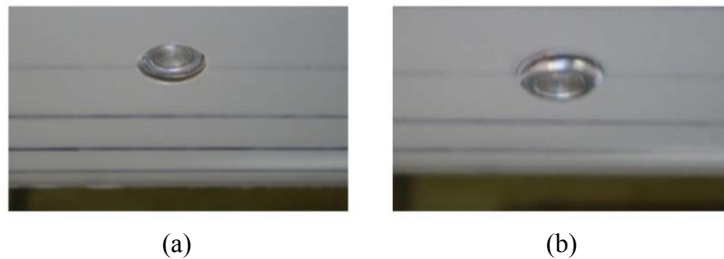
Figure 4-7: Wrong position of the sensor diaphragm: the diaphragm positioned 1.5 mm inside (a) and 1.5 mm outside (b) the cylindrical surface
