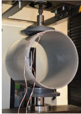
Figure 5-39: The test configuration for the compression test with cylinder C1
