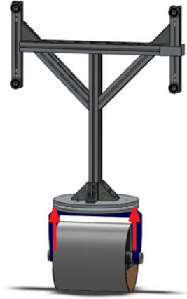
Figure 5-23: Illustration of the force introduction on the load cell combination
