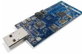
Figure 1.4. Tmote Sky sensor node
