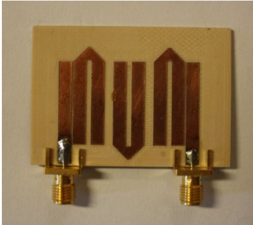
Figure 5.17: Realization of the hairpin filter for Case I with 5 mm feedline.
