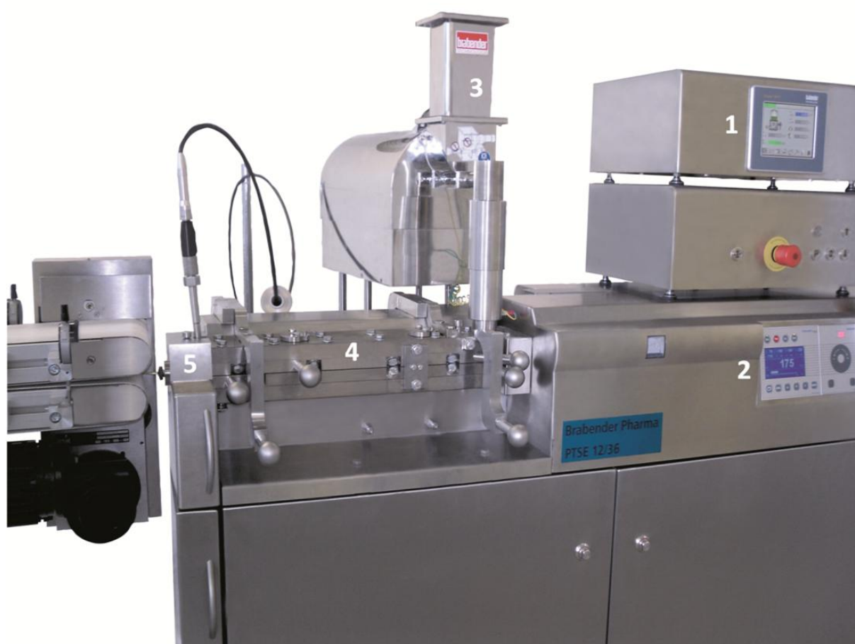
Figure 7.2. Experimental setup. 1) Extruder control panel, 2) Feeder control panel, 3) Feeder unit, 4) Extrusion barrel, 5) Extrusion die with implemented Raman probe.
