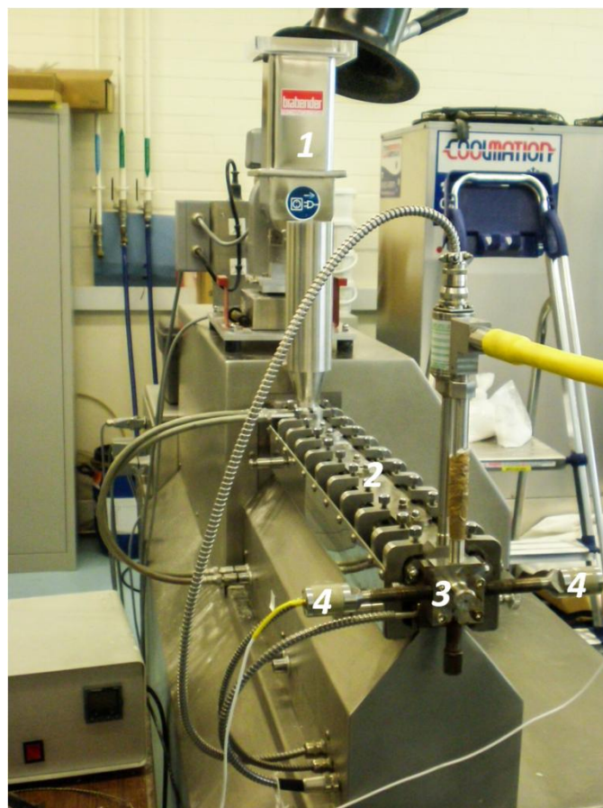
Figure 9.2. Experimental setup with longitudinal wave transducers mounted directly opposite one another in the extrusion die adapter. 1) Feeding unit, 2) extrusion barrel, 3) custom made die adapter, 4) ultrasound transducers.
