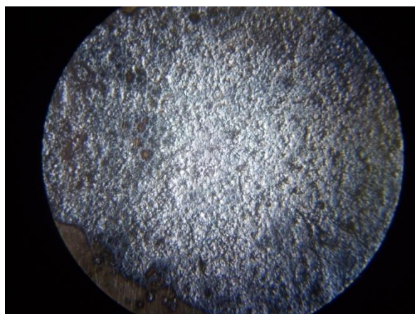
\text{MnO}_2\text{-Co}_3\text{O}_4\text{-CeO}_2 / \text{AlCe}_{0.2}\text{Zr}_{0.05}\text{O}_2 / \text{FeCr} alloy (Ca.10)
