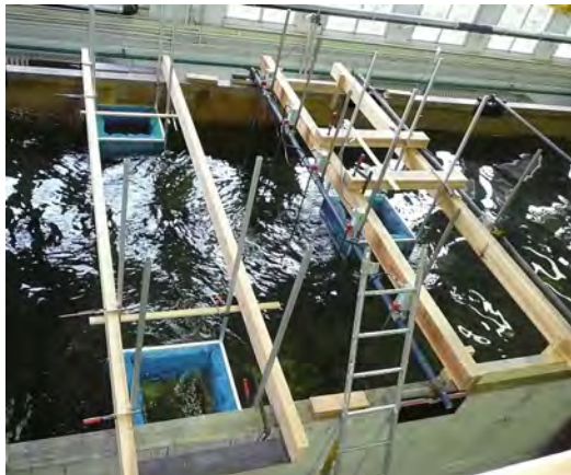
Figure 6.53: Plan view of a farm of 3 absorbing WECs (36 m (w) x 36 m (l) x 15 m (h) on scale 1/50) in the wave flume of Flanders Hydraulics Research
