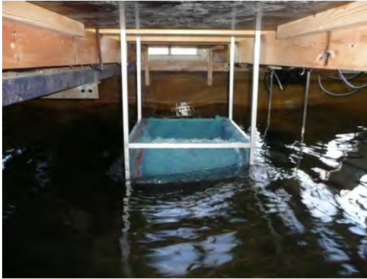
Figure 6.46: Side view of the WEC (36 m (w) x 36 m (l) x 15 m (h) on scale 1/50) in the wave flume of Flanders Hydraulics Research
