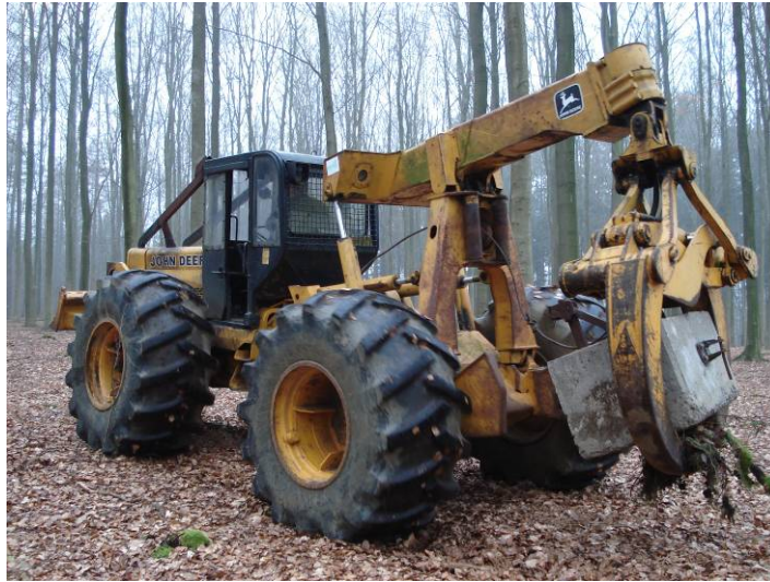
Figuur 2.1.4 John Deere grapple skidder JD640
