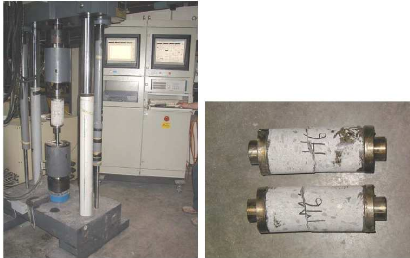
Figure 6.21: The test set-up to determine the pure tensile strength [BBRI, 2007]
