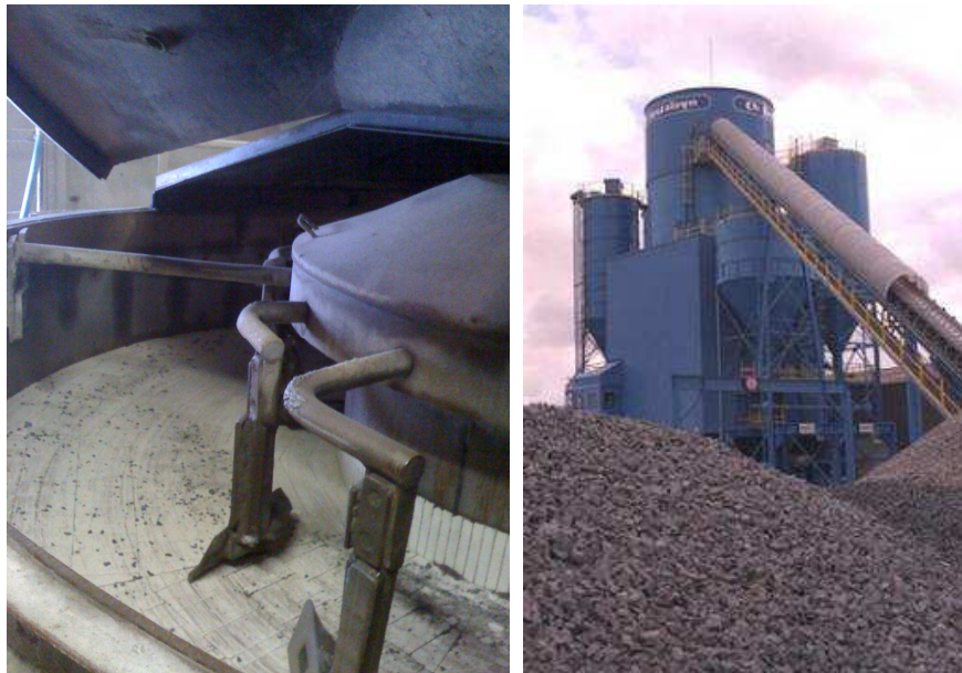
Figure 9.2: The concrete mixer with a capacity of 2 m 3 (left) and the mixing operation tower with the conveyer belt for transportation of the aggregates (right) at the Kesteleyn concrete factory
