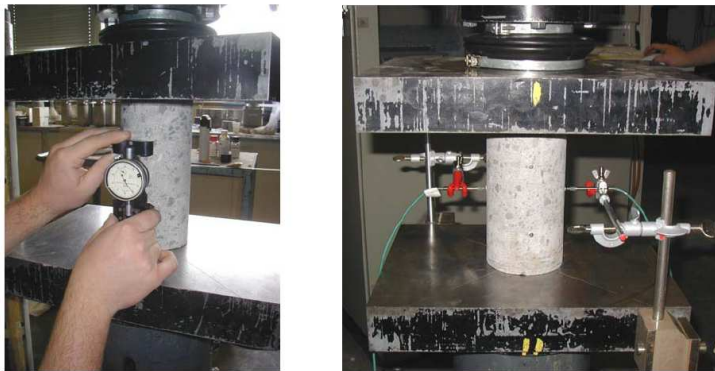
Figure 6.24: Determination of the modulus of elasticity (left) and Poisson's ratio (right) [BBRI, 2007]
