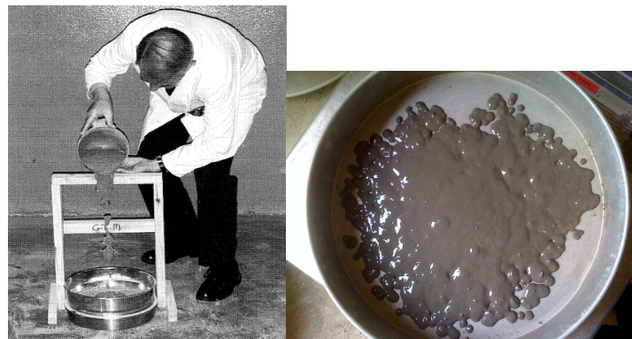
Figure 6.5: Sieve stability test: pouring of the SCC (left) and the amount of mortar fallen through the sieve (right)
