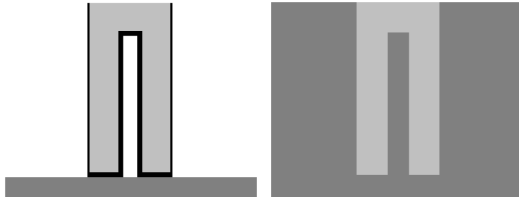
Figure 8.19a: Scheme of the reverse cast: standard situation (left) and casting in pit (right)
