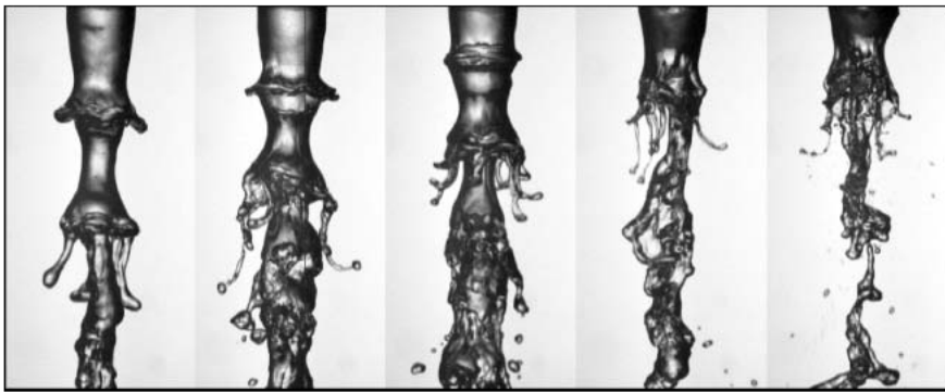
Figure 2.5: Snapshots of an 8-mm-diameter, slow (0.6 m/s) water jet destabilized by a coaxial fast air stream.; after [148]
