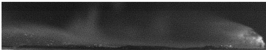
Figure 4.2: Typical front-light illuminated image for a q=10 circular injector jet; Mach 6 flow from right to left
