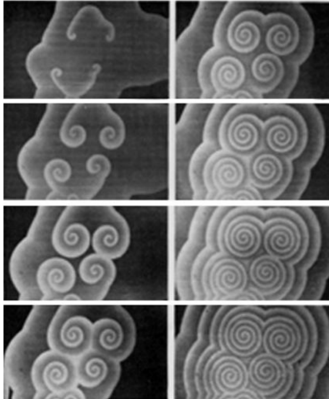
Figure 1.2: Spiral waves in the Belousov-Zhabotinsky reaction. Figure shows initiation of vortices or spiral waves in the BZ reaction. Taken from the paper by Zhabotinsky and Zaikin from 1971 [157].
