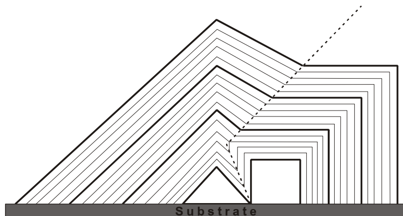
Figure 2.12: Overgrowth mechanism of faceted grains in which the grains with the most tilted facets with respect to the substrate overgrows the others. Figure adapted from Ref. [59].
