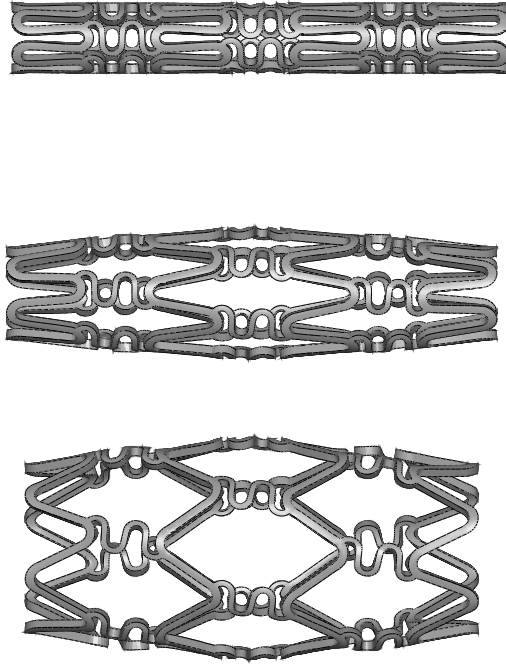
Figure 2.5: Illustration of pressure driven Cypher stent expansion (Neglect of the balloon). Top: no pressure; Middle: low pressure range; and Bottom: high pressure range.
