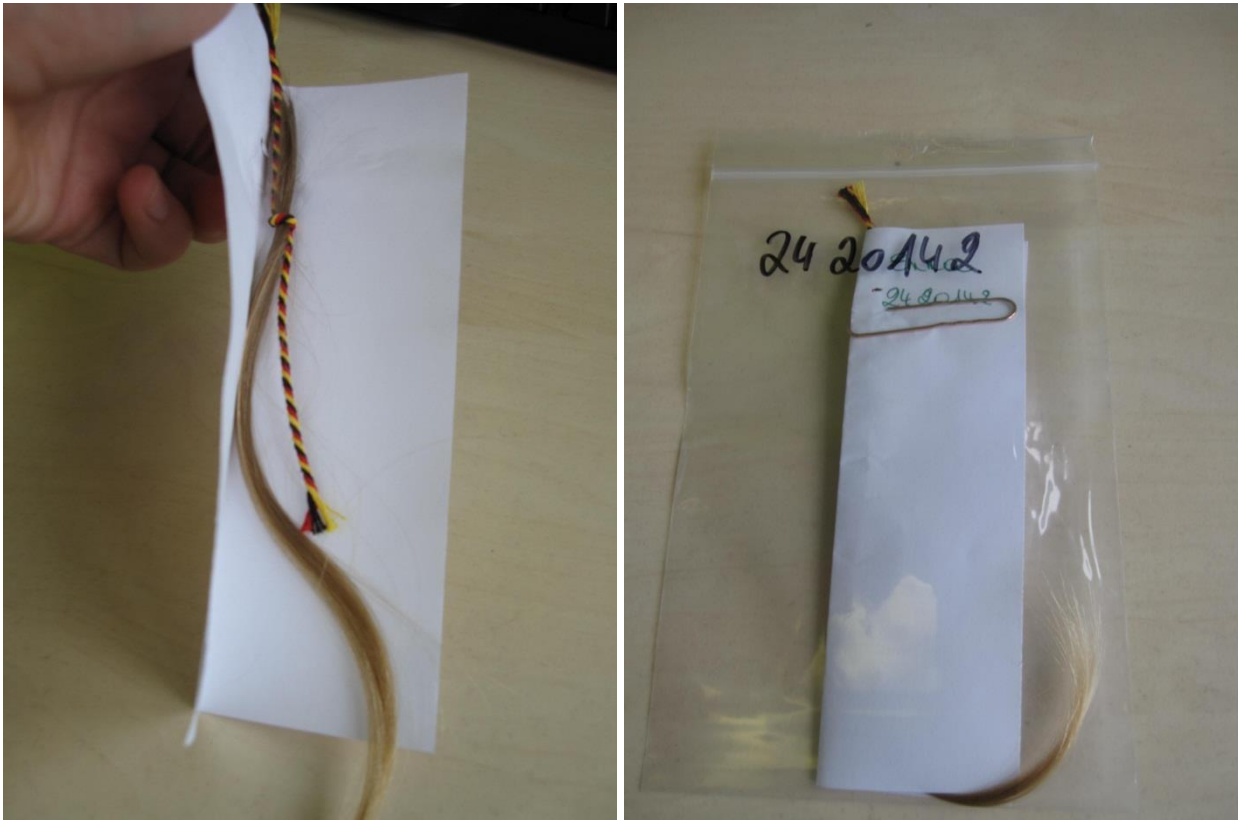
The strand of hair is fixed in a folded piece of paper using a paper clip at the side of the hair root (cord-side) without folding it. The hair sample is stored in a zip-lock bag with ID number.
