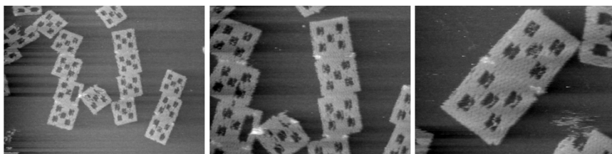
Figure 9.102: AFM images of the 5-well frame with (4 equivalents of) bridges annealed into it from 55°C overnight
