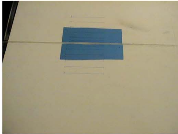
Figure 4. Set-up for the film measurements. Two radiochromic film pieces are positioned at both sides of the source catheter, which is embedded in the polystyrene slab. In this way it is possible to measure lateral profiles and a depth dose profile at the same time.
