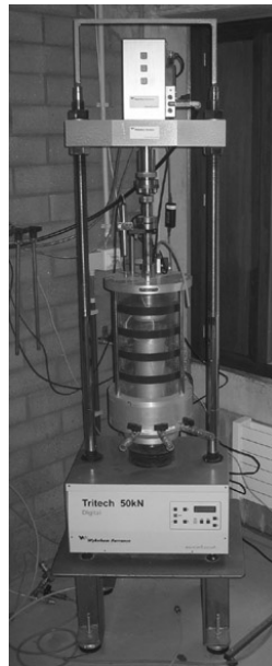
Figure 6.3-1: a) scheme and b) picture of loading frame and triaxial cell
