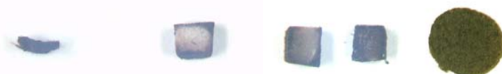
Figure 58 : Ink absorption of: left) silk non-woven, middle) three different precipitated scaffolds and right) salt-leached scaffold.
