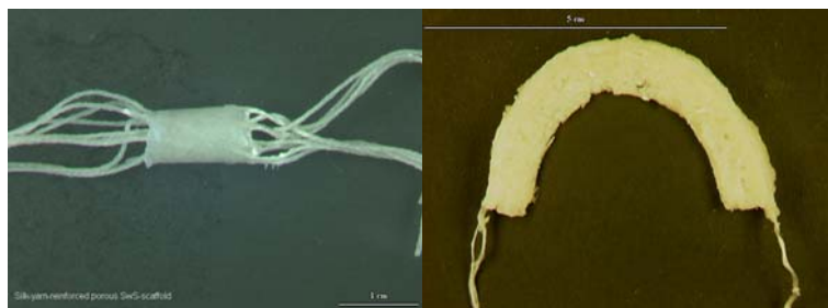
Figure 66 : Cartilage and meniscus silkworm silk scaffold reinforced with silk yarns to improve the tensile properties.
