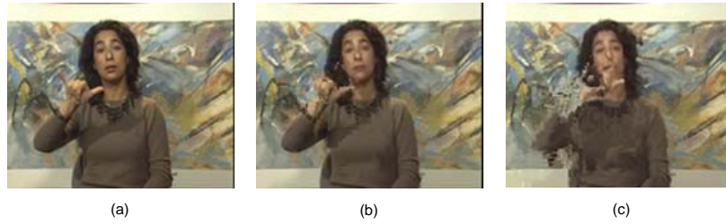
Figure 3.5: Example of SNR scalability using data partitioning, shown for frame 75 of the Silent test sequence: (a) no data partitioning; (b) disposal of partition C; and (c) disposal of partition B and C (showing ghosting artifacts). A value of 5 is used for the IMBR parameter.
