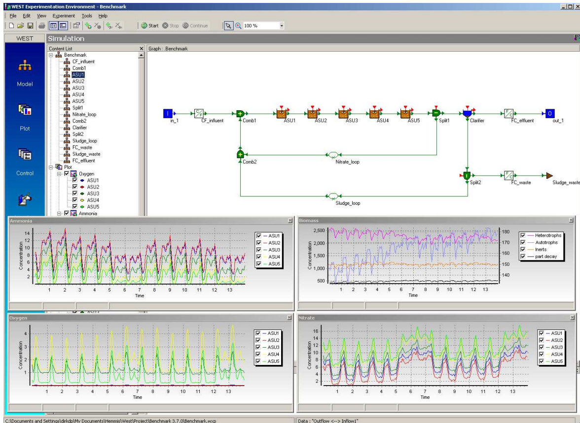
Figure 2.2: Screen shot of the WEST experimentation environment. Beside the simulation output, a graphical representation of the plant model is also shown.
