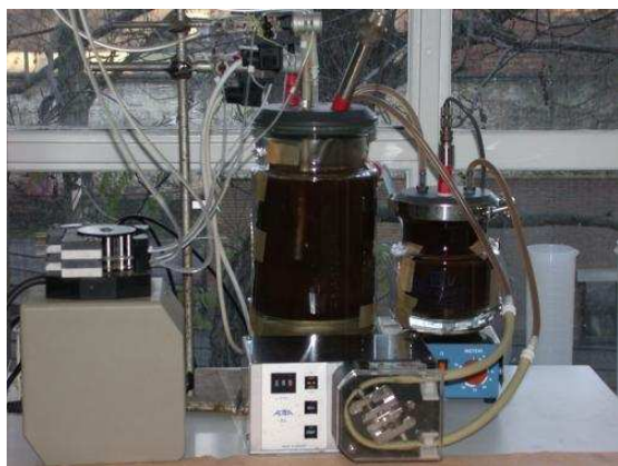
Figure 7.2: Picture of the hybrid respirometer installed at the BIOMATH lab.
