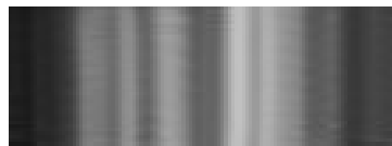
Fig. III.6 (identical to Fig. VII.B_4): This enlarged Schlieren image of a bounded ultrasonic beam, shows a fringing pattern that enables the determination of the fiber direction in composites.
