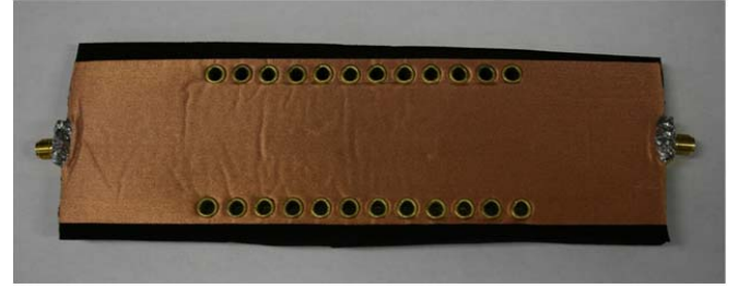
Fig. 9. Proposed SIFW interconnection: (a) structure (dimensions in mm: l_t=28.7 , w_t=19.6 , w_m=8.5 , h=3.94 , s=8 , d=4 , g=4 , w=41.2 , l=96 ), (b) photograph.
