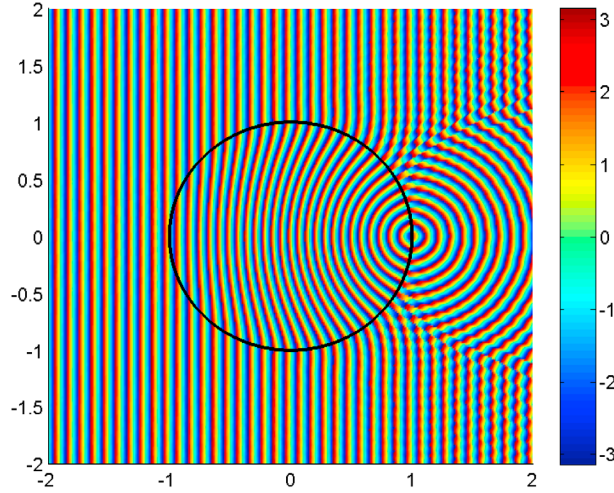
Figure 1b. Phase of the total electric field over the cross section. The flat phase fronts of the plane wave are gradually bent toward the focal point. The focal point of the Luneburg lens is E_0 = 1 \frac{\text{V}}{\text{m}} , R = 1 m.
