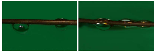
FIG. 9. Wettability of the PI dielectric layer before (left) and after (right) corona treatment
