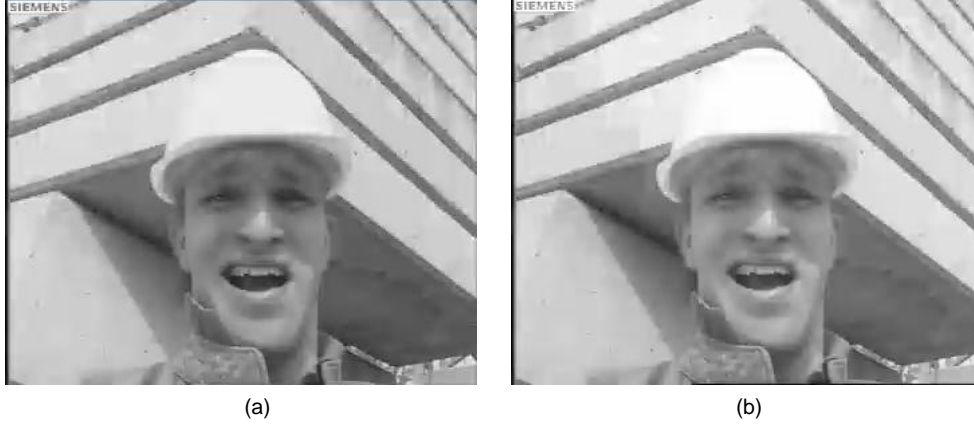
Figure 18: Impact of eliminating the clipping of reconstructed values on the decoded output for an intra-coded video sequence (Foreman, CIF) encoded with JM 18 using one slice. (a): decoded using a standard-compliant decoder, (b): decoded without clipping using the proposed restricted two-dimensional algorithm; notice how the error starting above the helmet propagates to the bottom right.
