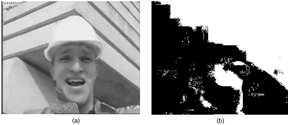
Figure 19: Impact of eliminating rounding of reconstructed values on the decoded output for an intra-coded video sequence (Foreman, CIF) encoded with JM 18. (a): decoded without rounding using the proposed restricted two-dimensional algorithm, to the authors visually indistinguishable from the correctly decoded image, (b): view of error introduced by neglecting the rounding operations (black and white areas show correctly and faulty decoded samples respectively).
