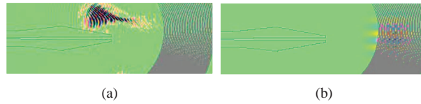
Fig. 4. 3D FDTD simulations showing (a) the refocusing of the reflection using an over-saturated electrical field (Media 1) and (b) waveguide coupling when excited from the fiber (Media 2) ( \sigma = 90^\circ , \phi = 15^\circ )
