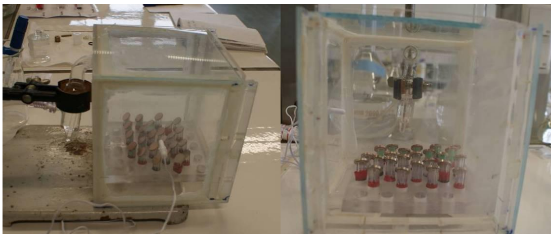
Figure 1. Photographs of the spray chamber for the corrosion tests.
