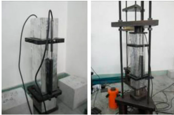
Figure 3. Shrinkage (left) and creep (right) test setup.
