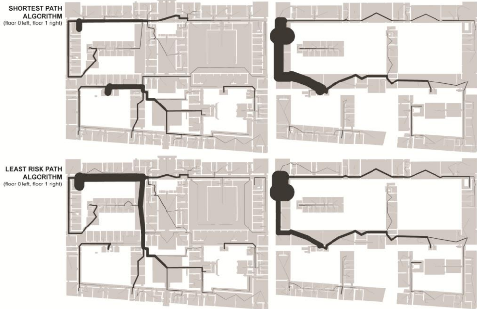
Fig. 5: Path use of the shortest path and least risk path algorithm (source node 1086)
