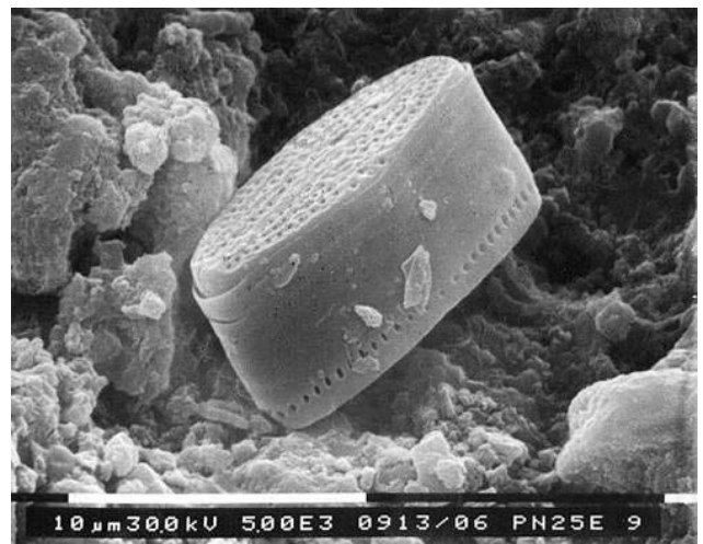
Fig. 14 - Diatom algae found in the same sample as Fig. 9 taken from a concrete structure placed in a hot and dry environment.
