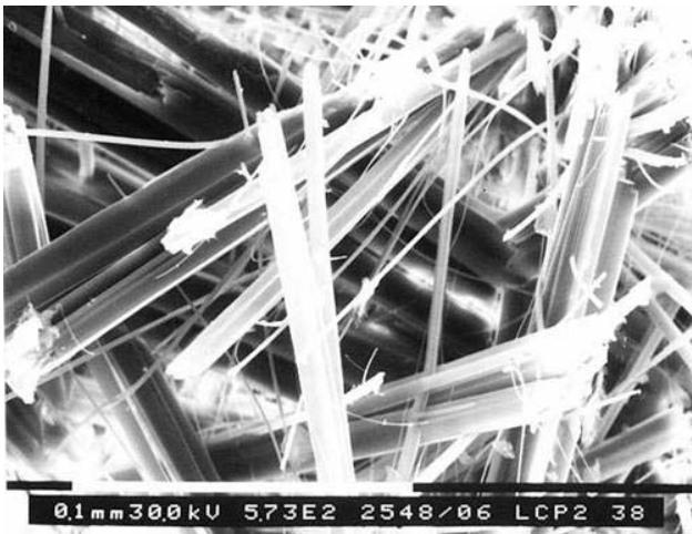
Fig. 17 - Ettringite observed in a concrete apparently sound but where it was observed deteriorated micaceous solubilised calcium carbonates and portlandite.
