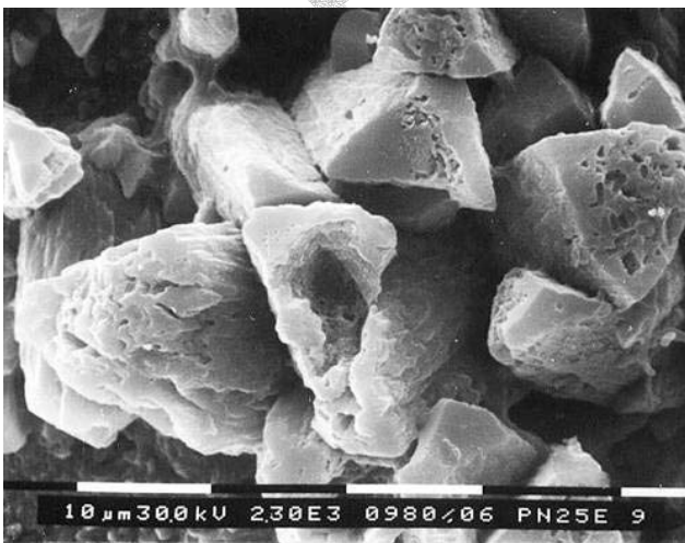
Fig. 13 - Solubilised calcium carbonates observed in a concrete where Cladosporium and protozoa were also present.
