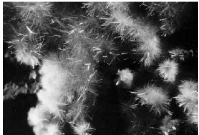
Fig. 12 - Crystals formed on concrete through action of bacterially produced organic acids (lactic and acetic acids).
