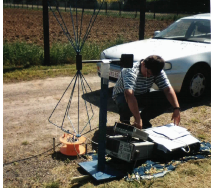
Fig. 8: Calibrated antenna set-up with a pulse generator.
