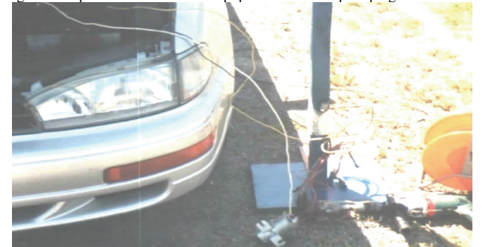
Fig. 10: Detail of the set-up of the measurement equipment with the spark plug.
